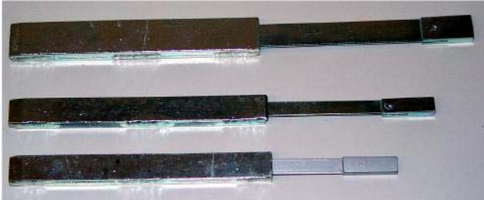
Prevents wedges from breaking or bulging while being driven into place. Steel shell construction with a steel driver. Shell length 6".
